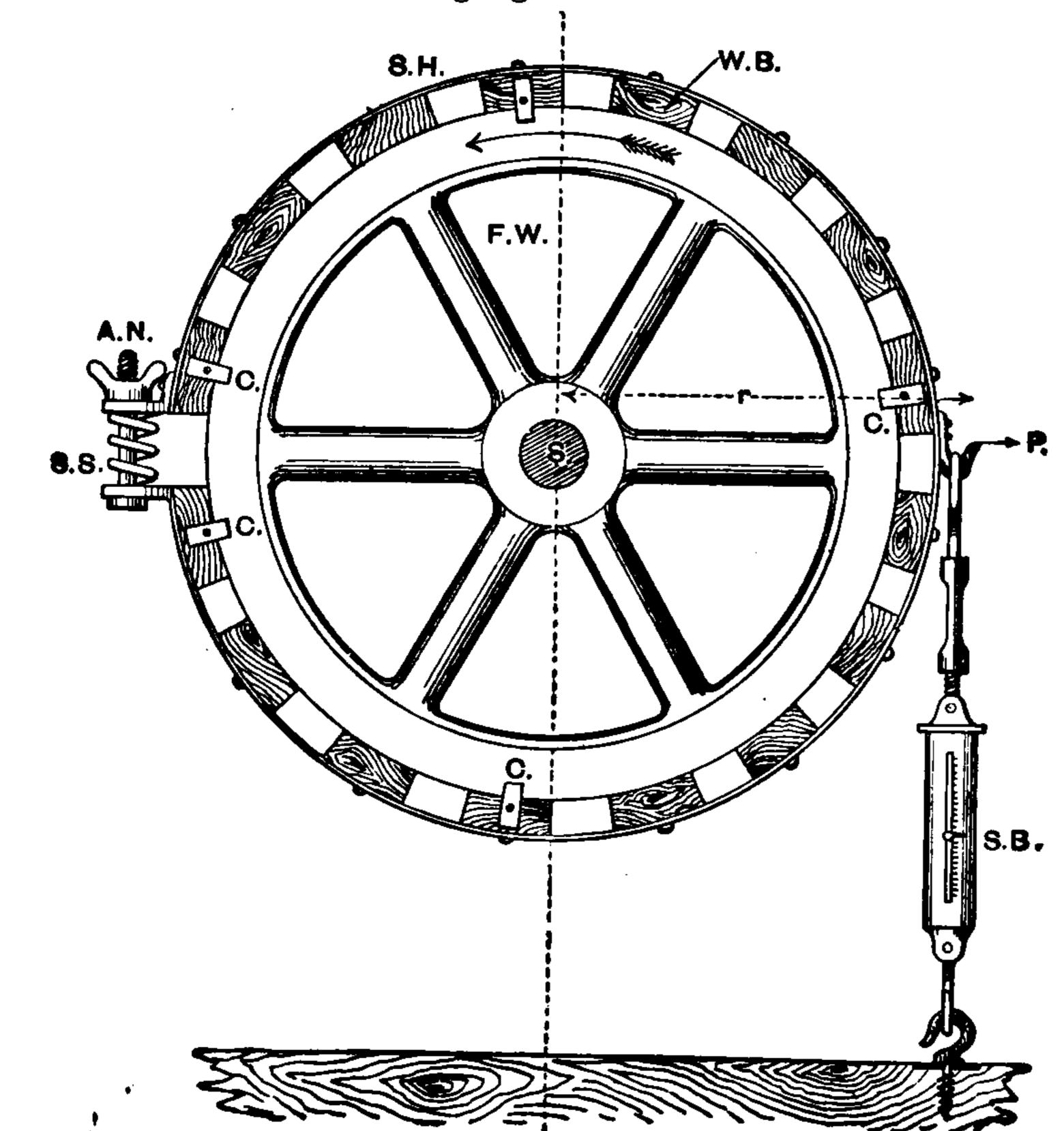
Here the balance weight and ram nuts are done away with, in favour of a steel hoop or strap, SH, to which are fitted wooden blocks, WB, with spaces, of say 2 inches or so intervening between them, surrounding the fly-wheel, FW, keyed on the crank shaft, S. Clips, C, made of iron or steel, keep this brake strap fair on the fly-wheel, and thus prevent it from sliding to one side more than another.
