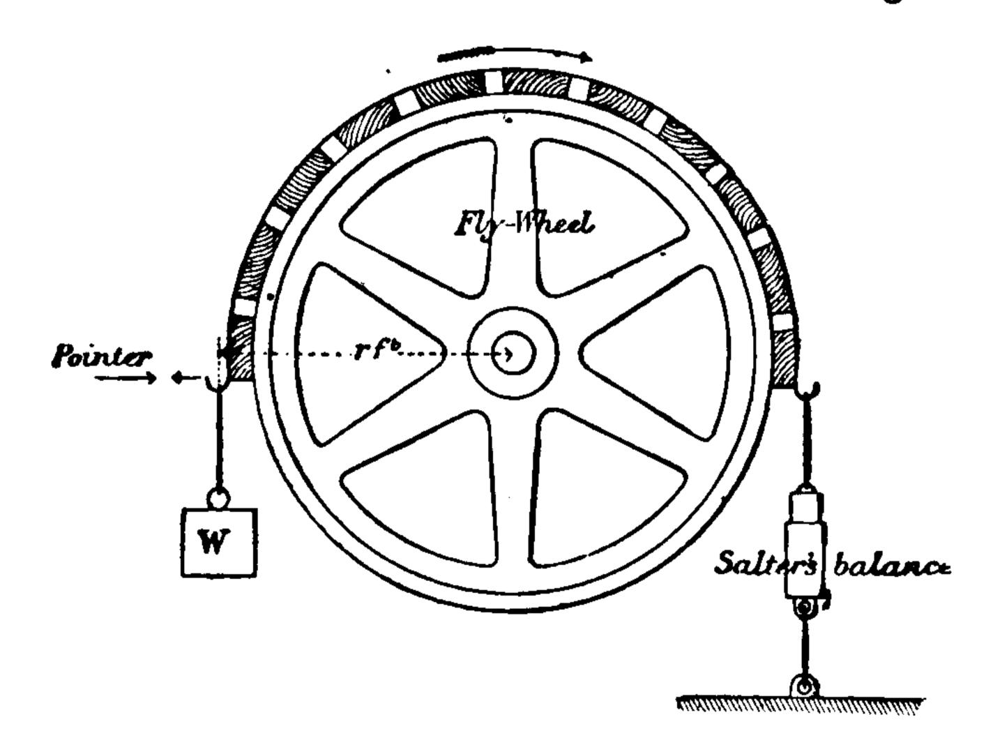
adopted instead, which gave fairly good results with the gasengine, developing 13.6 brake H.P. The chief objections, however, to it were:—1. That even for that small power, it was necessary to have two brakes, one brake upon each fly-wheel.
